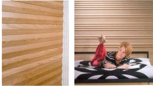
**BASF** has developed pigment preparations for through-colored medium density fiberboard (MDF). BASF calls this product "Design-MDF". The brilliant, vivid colors bring out the wood fibers and give the impression of a natural material.
